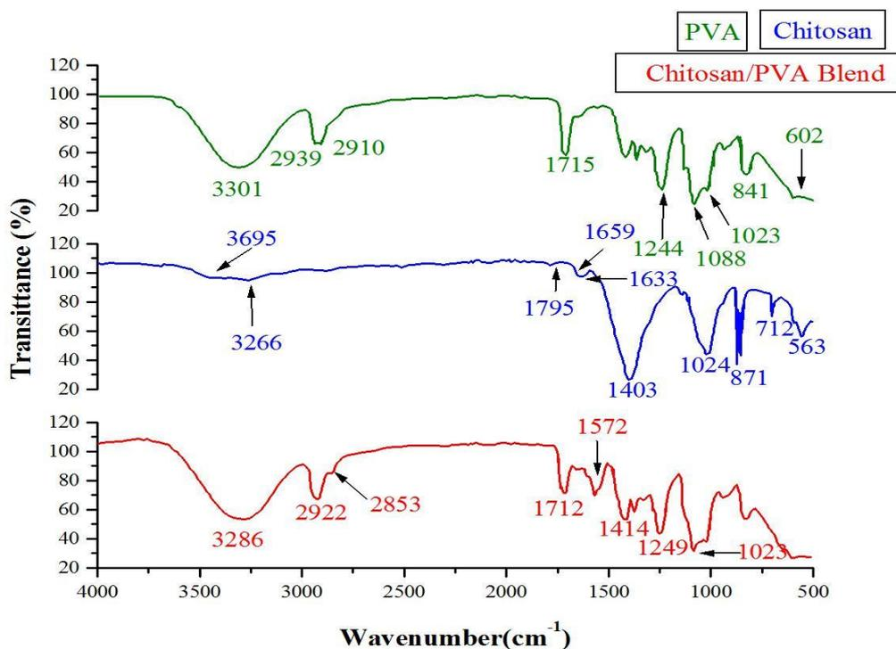
Fig. 6: FTIR Spectrum of Chitosan (blue), polyvinyl alcohol; PVA (Olive), and Chitosan/PVA blend (1:1) (Red)
