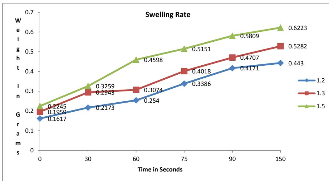
Fig 4: Swelling kinetics of composite film formulations of glutaraldehyde cross-linked chitosan-PVA and chitosan-PVA up to 150 second at 37°C
