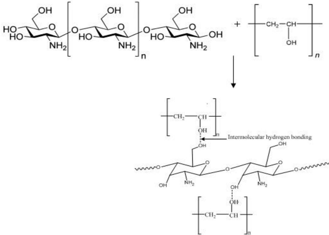
Scheme 2: Intermolecular hydrogen bonding between chitosan and PVA
