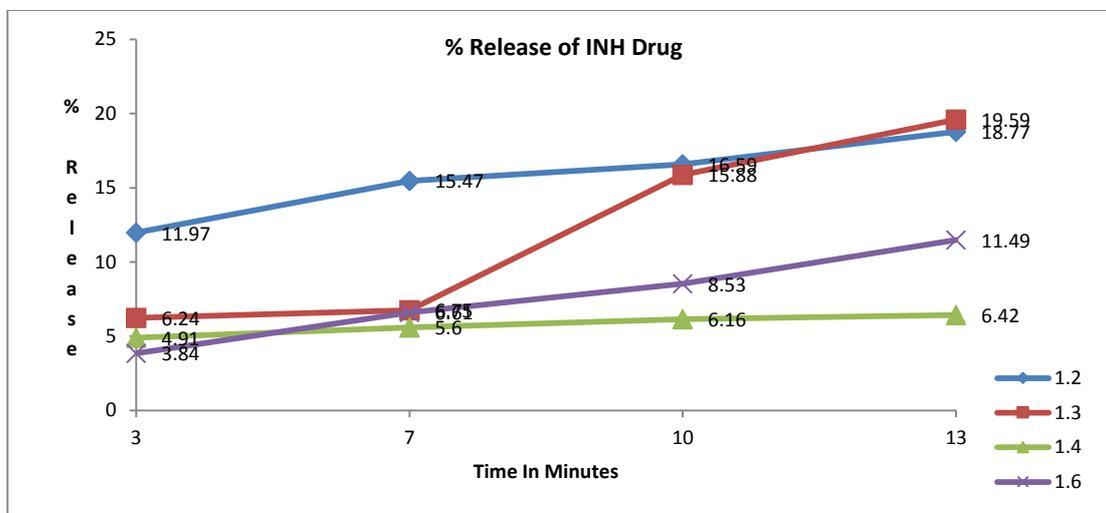
Fig. 5: Percentage (%) release of INH drug of Chitosan-PVA film formulations up to 13 min
